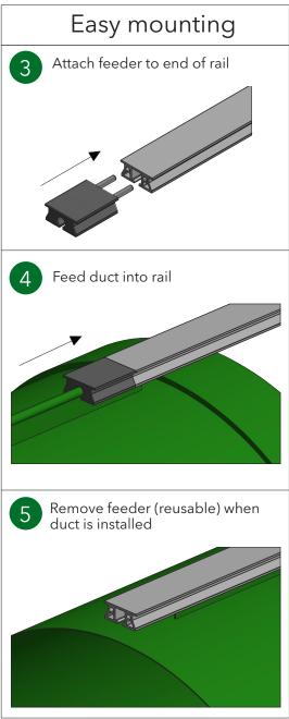
Install rail system according to drawings and enclosed mounting instructions
